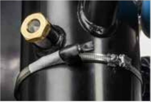
Oil heater → Prevents condensation formed due to intermittent use by maintaining a constant oil temperature while unloading/idle.
